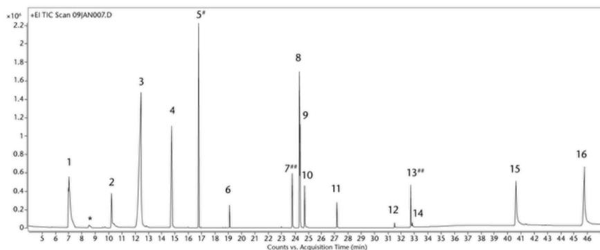
Figure 4. Typical chromatogram, GC/MS system suitability mixture. See [Table 4](#) for peak labeling. \*, system peak; #, internal standard peak (2-fluorobiphenyl); ##, secondary internal standard peaks (caffeine-(trimethyl-<sup>13</sup>C<sub>3</sub>) and Tinuvin 327).
