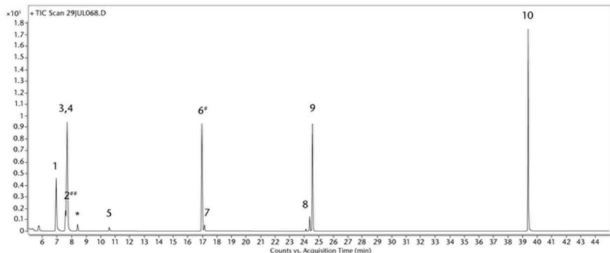
Figure 3. Typical chromatogram, HS-GC/MS system suitability mixture. See [Table 3](#) for peak numbering. \*, system peak; #, internal standard peak (toluene-D<sub>8</sub>); ##, secondary internal standard peak (acetone-D<sub>6</sub>).
