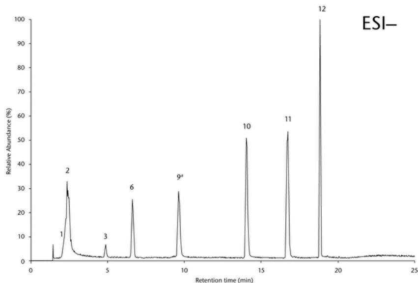
Figure 8. Typical chromatogram, LC/MS-ESI- system suitability mixture. Refer to [Table 6](#) for peak numbers. #, internal standard peak (terephthalic-D<sub>4</sub> acid). Note that the actual chromatographic run ends at 29.5 min, followed by re-equilibration.
