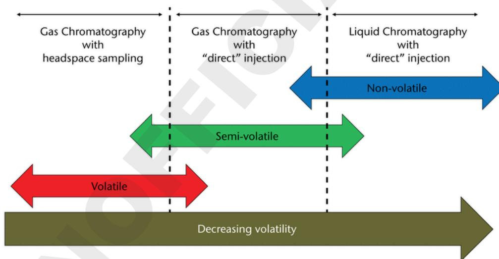
Figure 1. Application of chromatographic methods in extractables and leachables screening.
