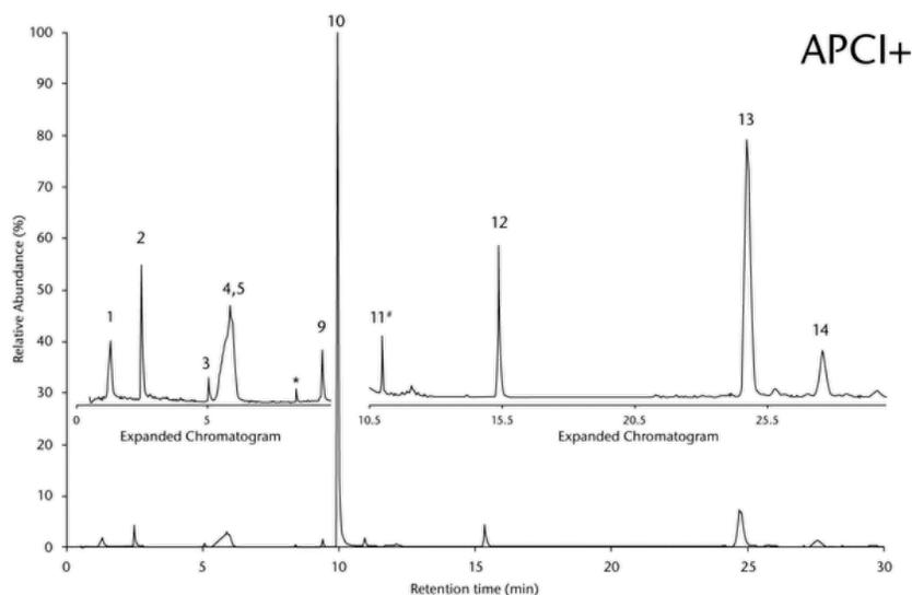
Figure 5. Typical chromatogram, LC/MS-APCI+ system suitability mixture. See [Table 5](#) for peak labeling. \*, system peak; #, internal standard peak (Tinuvin 327). Note that the actual chromatographic run ends at 29 min, followed by column rinsing and re-equilibration.
